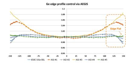
AEGIS Allows for Ge% Profile Tuning at the far wafer edge (1.2mm)
