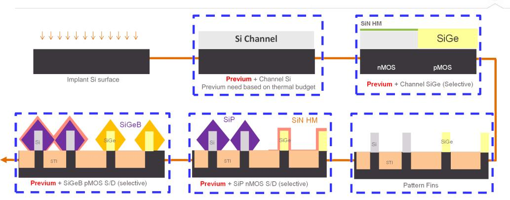
Simplified Logic Process Flow Highlights the Need for Multiple Integrated Previum Surface Cleaning Steps
