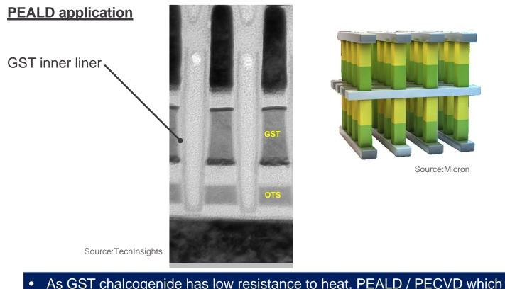
• As GST chalcogenide has low resistance to heat, PEALD / PECVD which enables low temperature film deposition is widely used.
