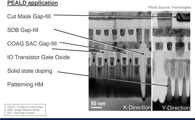
Maintaining POR position in oxide layers. Adding high quality oxideDevice shrinkage increases demand for PEALD layers
