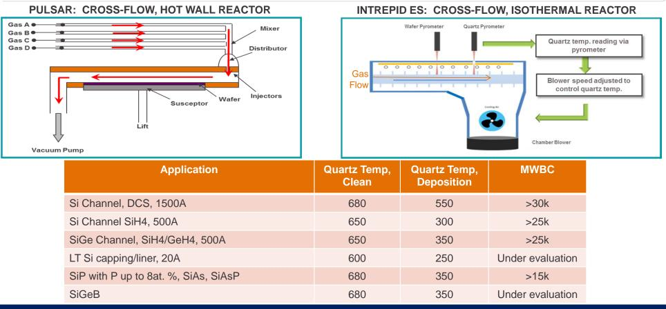
Controlling quartz temperature during deposition and chamber cleans has proven to show excellent WTW performance and long MWBC cycles
