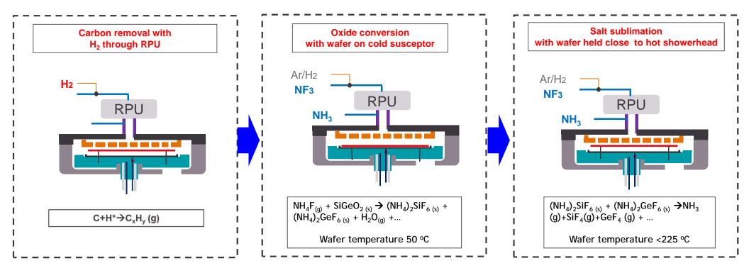
**Previum Process Optimized for Wafer Surface Cleaning at Low Temperatures**
